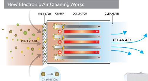
Particulate carried in the exhaust air enters the cell and is charged by the ionizing blades. The charged contaminants then travel into the collector stage where similarly charged plates repel them, and they adhere to the ground plates, where the collected effluent drains off or is washed by the auto wash system periodically.
