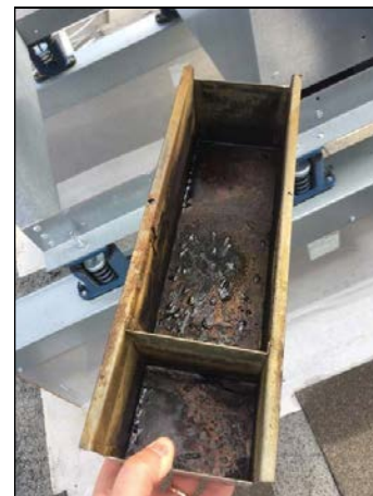
Grease trough (cleaned 4 weeks earlier)
